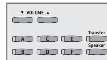
For the purposes of programming speed dial numbers, the programmable keys are known as **A**, **B**, **C**, **D**, **E** and **F** and are defined below.
