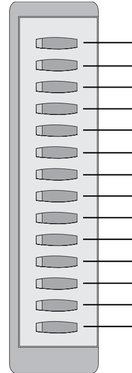
**14 PROGRAMMABLE KEYS WITH RED LIGHTS** Used to call stations directly, to indicate busy conditions of other stations, for One Touch dialing and many other system features.
